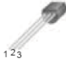
78L12, Voltage Regulator, TO-92
